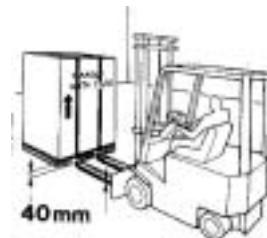
For moving the packed unit to site use a fork lift with forks no thicker than 40 mm.
