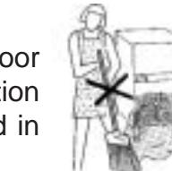
During the cleaning of the floor near the machine pay attention that dust does not get sucked in the unit by the fan motor.
