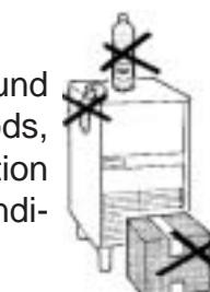
Do not place on top and around the ice maker any sort of goods, which can limit proper ventilation and jeopardize hygienic conditions.
