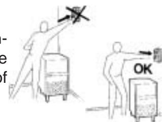
The electrical disconnect switch must be within hand reach of the installed machine.
