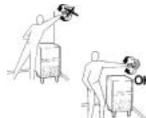
The water shut-off valve must be within hand reach of the installed machine.
